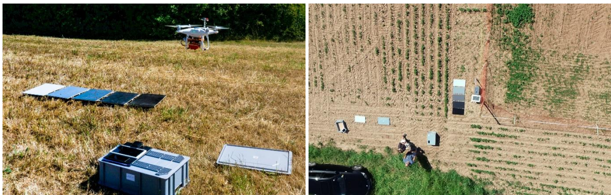
Figure 21: Reflectance target used for empirical line correction.
